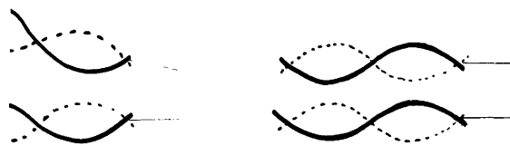
Fig. 3. Mechanism proposed in order to form the curved layers of clusters. The normal close-packing arrangement of double helices is shown to the right, and the proposed translation in order to account for a change in the direction of the helical axes is shown to the left.
